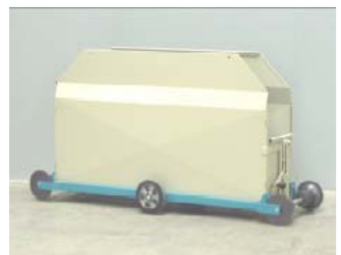
Transportation cart with bottom unloader for peppers
